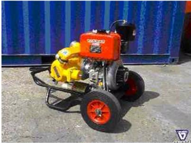
Diesel-driven Spate Pump (Slurry) with pumping capacity of 30 KL/Hour
