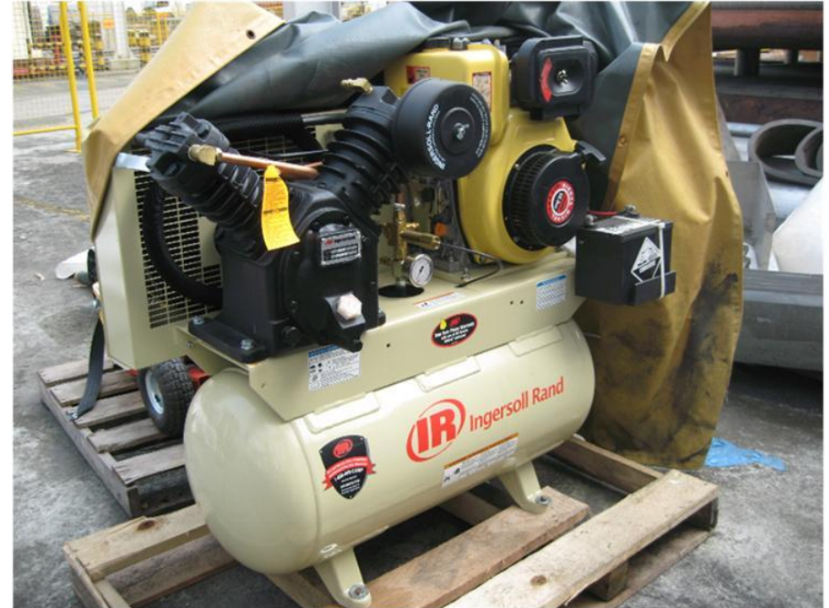
Diesel driven Air Compressor to drive Pneumatic Eqpt and Tools
